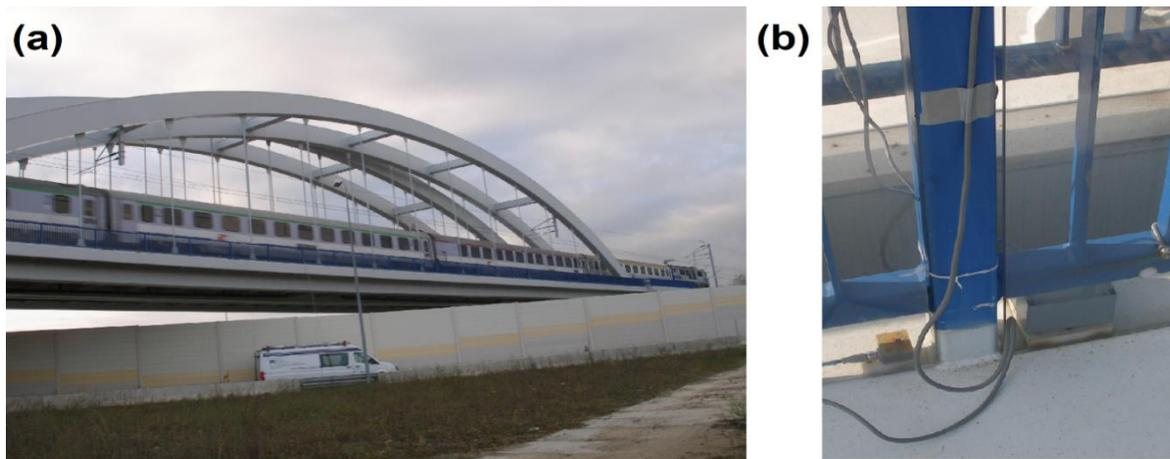
**Figure 3.** Monitoring of the dynamic deflection under service load; (a) view of the bridge; (b) accelerometer and one of the three inclinometers and location at the bridge deck.
