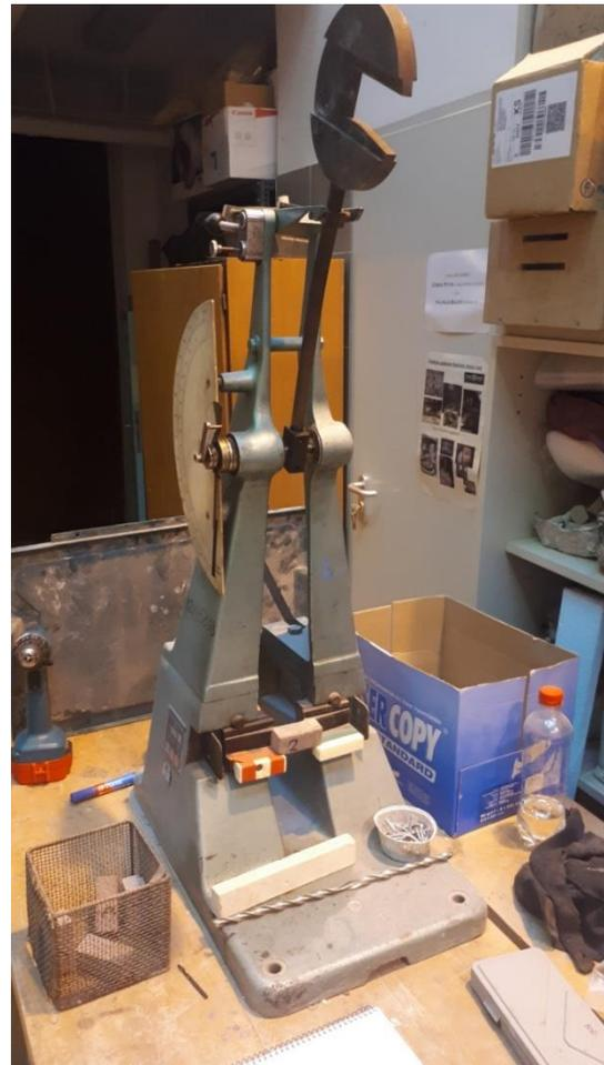
**Figure 1.** Theoretical arrangement of the Charpy hammer test and in the laboratory
