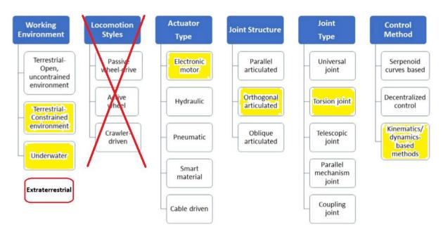
**Figure 1**. Classification methods of snake robots (figure after [3]). *Arm-Z* belongs to the class of: constrained, various environments, no locomotion, electric motor, orthogonal, torsion joints, kinematic based control manipulators.
