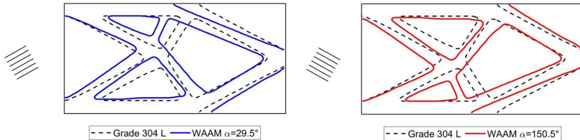
Figure 3. Simultaneous design of the topology and the printing direction for WAAM: optimal results (continuous lines) compared to conventional design with isotropic assumption (dotted line).
