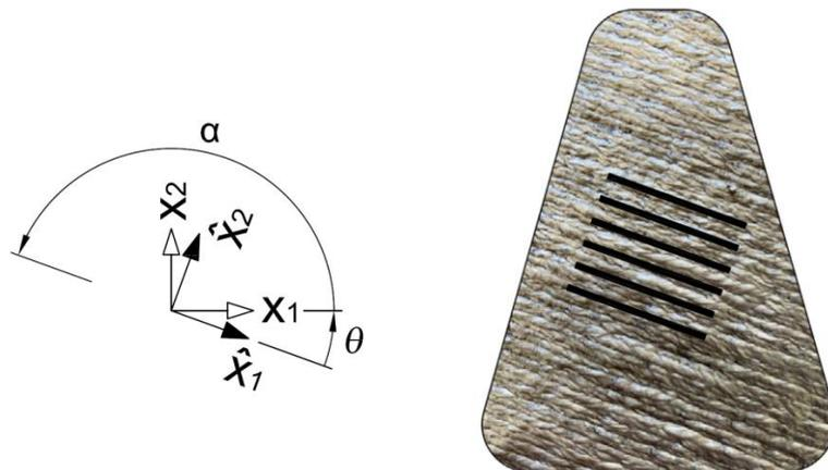
**Figure 1.** Orientation of the printed layers for an object framed in the general reference system with axes  $x_1$  and  $x_2$ .  $\hat{x}_1$  and  $\hat{x}_2$  are the symmetry axes of the alloy, i.e., the longitudinal direction (L) and the transversal direction (T), respectively.
