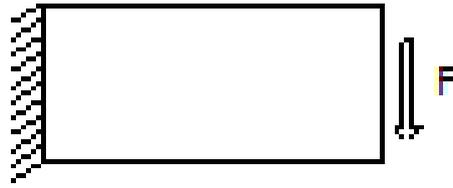
Figure 2. A cantilever beam.
