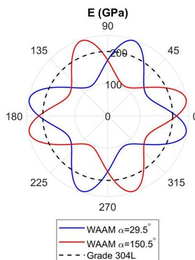
Figure 4. Polar plot of the Young's modulus of WAAM-produced stainless steel for the two optimal printing directions. The angular coordinate identifies the direction along which the modulus is given with respect to  $x_1$ . The value for Grade 304 stainless steel is reported for comparison.
