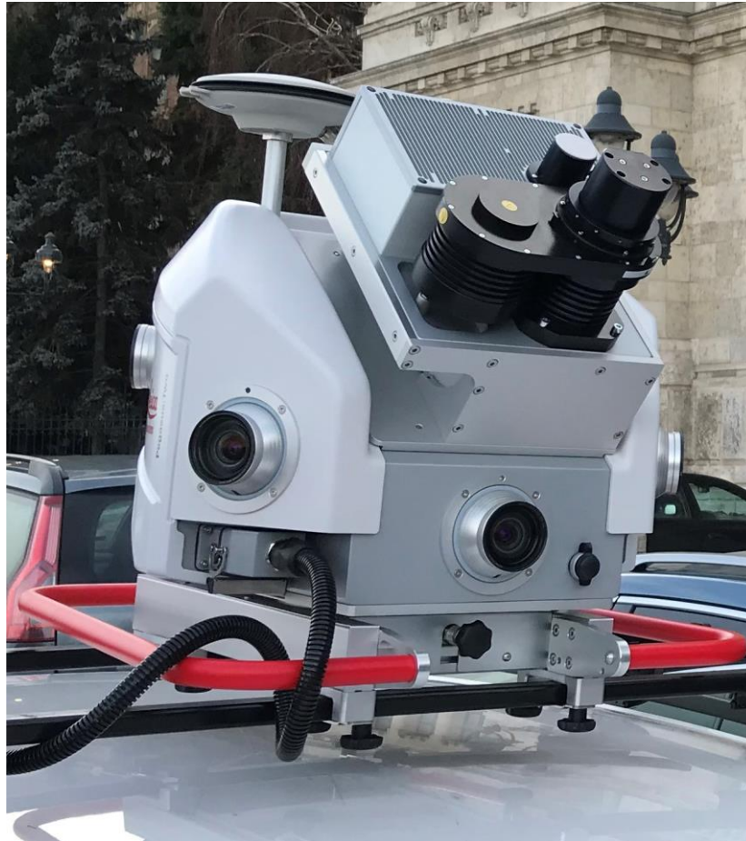
Figure 3. A Leica Pegasus Two mobile mapping system mounted on top of a car
